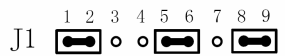
(c) CW/CCW mode and effective when the opto-coupler of the fixed level in conducting state
