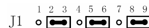
(d) CW/CCW mode and effective when the opto-coupler of the fixed level in off state
